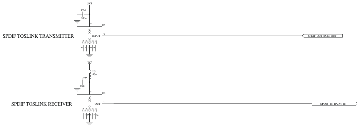
Figure 10.5: Example Circuit for SPDIF Interface (Optical)
