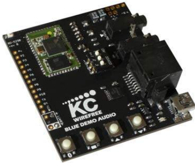
BD-5190 Blue Demo Class 1 Hi Power Audio Board BD-5290 Blue Demo Class 2 Audio Board
